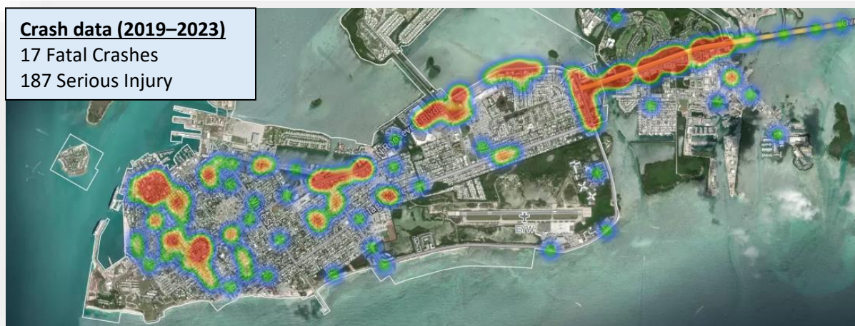
Figure 6. Preliminary hotspot analysis based on the five-year crash data from Signal 4 Analytics
