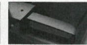
Rear console plate. Interfaces with front console mounting plate and extends through 2nd-row occupant area to seat bottom; acting as wiring conduit on top of transmission tunnel.
