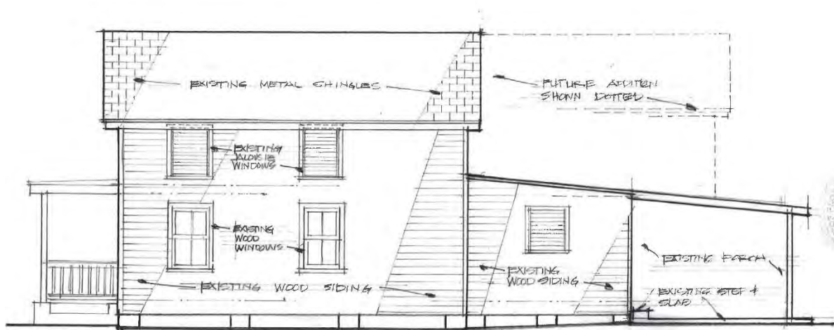
Existing south elevation with second story addition drawn with dotted lines.
