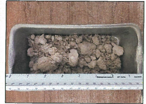
CEMENTED OOLITIC LIMESTONE W/ SILT [TB-1 @ 8 FT]
