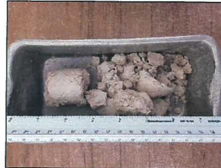
CEMENTED OOLITIC LIMESTONE [TB-1 @ 18 FT]
