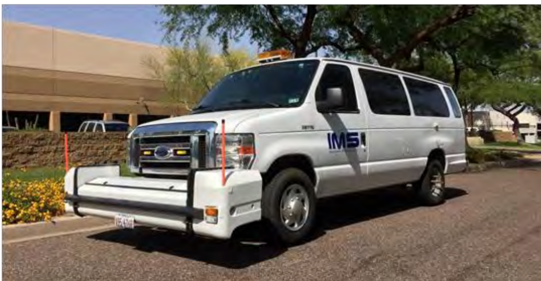
Figure 4 – Laser Road Surface Tester (RST)
