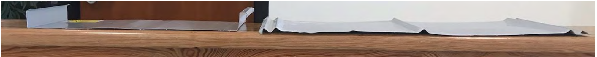
Proposed standing seam to the left vs. 5 v-crimp to the right profile view.
