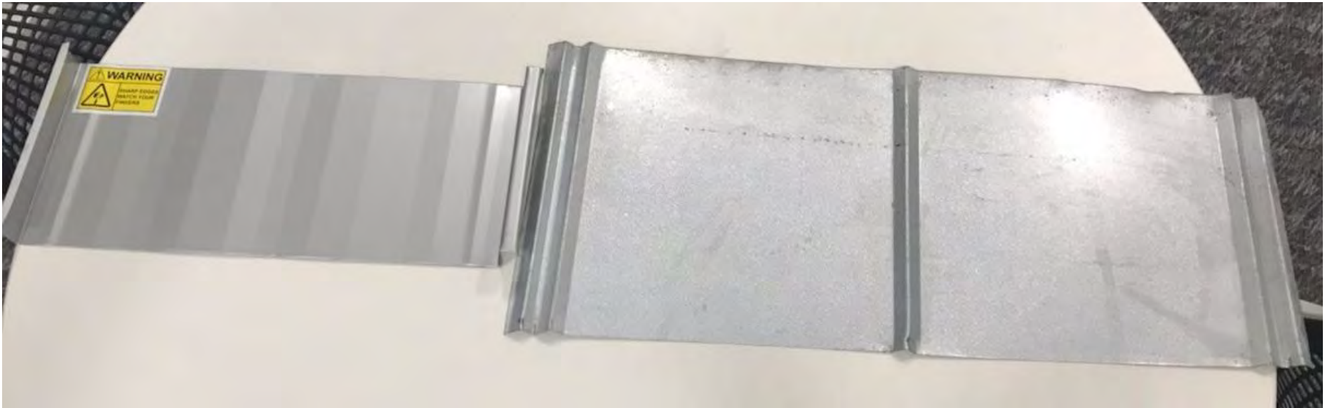
Proposed standing seam to the left vs. 5 v-crimp to the right upper view.
