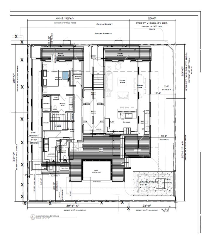
Close up of Rear Set Back dimensions. Same as previous plans. Nothing changed, except the way the rear setback is counted. The new pool deck was lowered to 28 1/2". This now makes the pool an accessory structure, will not be included in the building coverage.
