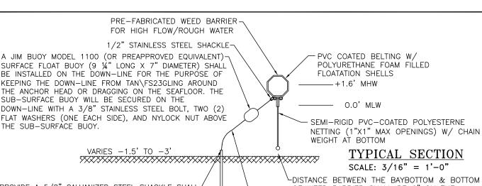
PROVIDE A 5/8" GALVANIZED STEEL SHACKLE SHALL-SECURE THE DOWN-LINE TO THE GALVANIZED ANCHOR HEAD. THE DOWN-LINE WILL BE LOOPED AT THE AN\FS23CHOR END, CONNECTED TO ITSELF WITH A 3/8" STAINLESS STEEL BOLT, TWO (2) FLAT WASHERS (ONE EACH SIDE), AND A NYLOCK NUT. THE LOOPED END OF THE DOWN-LINE WILL BE COVERED WITH 3 1/2" X 12" LONG CAN\FS23VAS FIRE HOSE, AND HELD IN PLACE WITH AT LEAST TWO HEAVY DUTY CABLE TIES.
