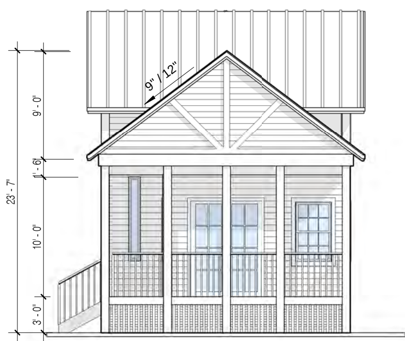
6 C2 - Alternate Side Elevation
