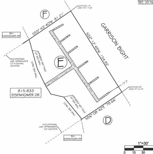
NORTH ARROW IS REFERENCED TO GRID NORTH, BASED ON THE 1990 ADJUSTMENT OF THE NORTH AMERICAN DATUM OF 1963 (NAD 83/90), FLORIDA STATE PLANE COORDINATE SYSTEM (TRANSVERSE MERCATOR PROJECTION), EAST ZONE (0901).
