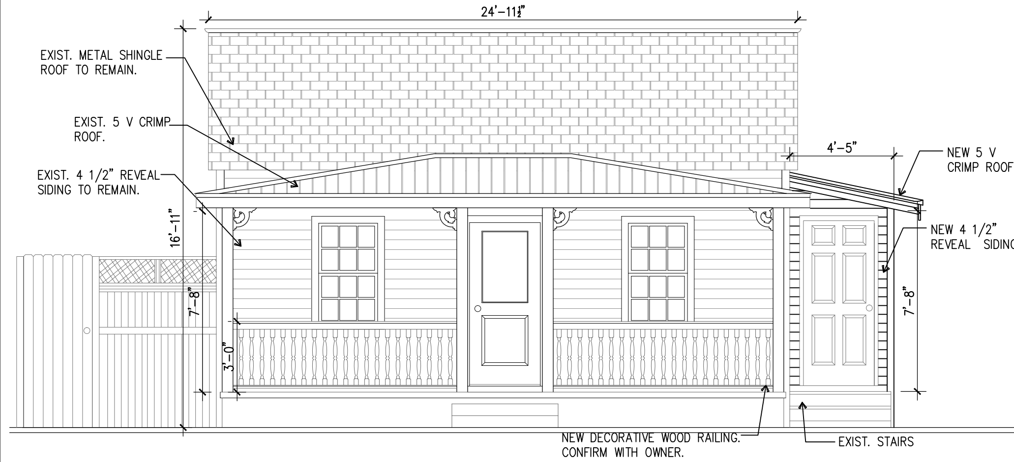
4 PROPOSED FRONT ELEVATION A-2 SCALE: 1/4"= 1'-0"
