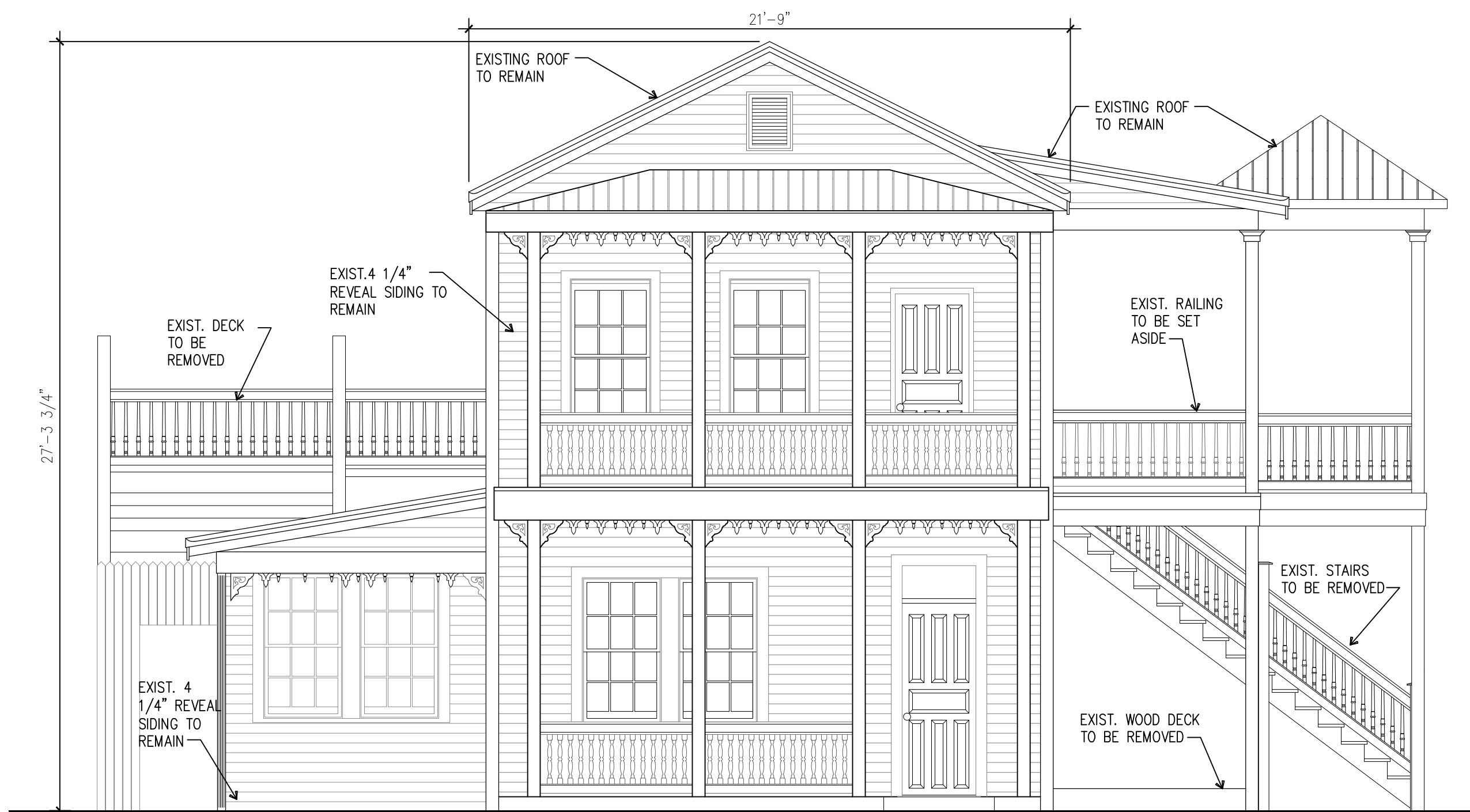
2 EXISTING FRONT ELEVATION A-201 SCALE: 1/4" = 1'-0"
