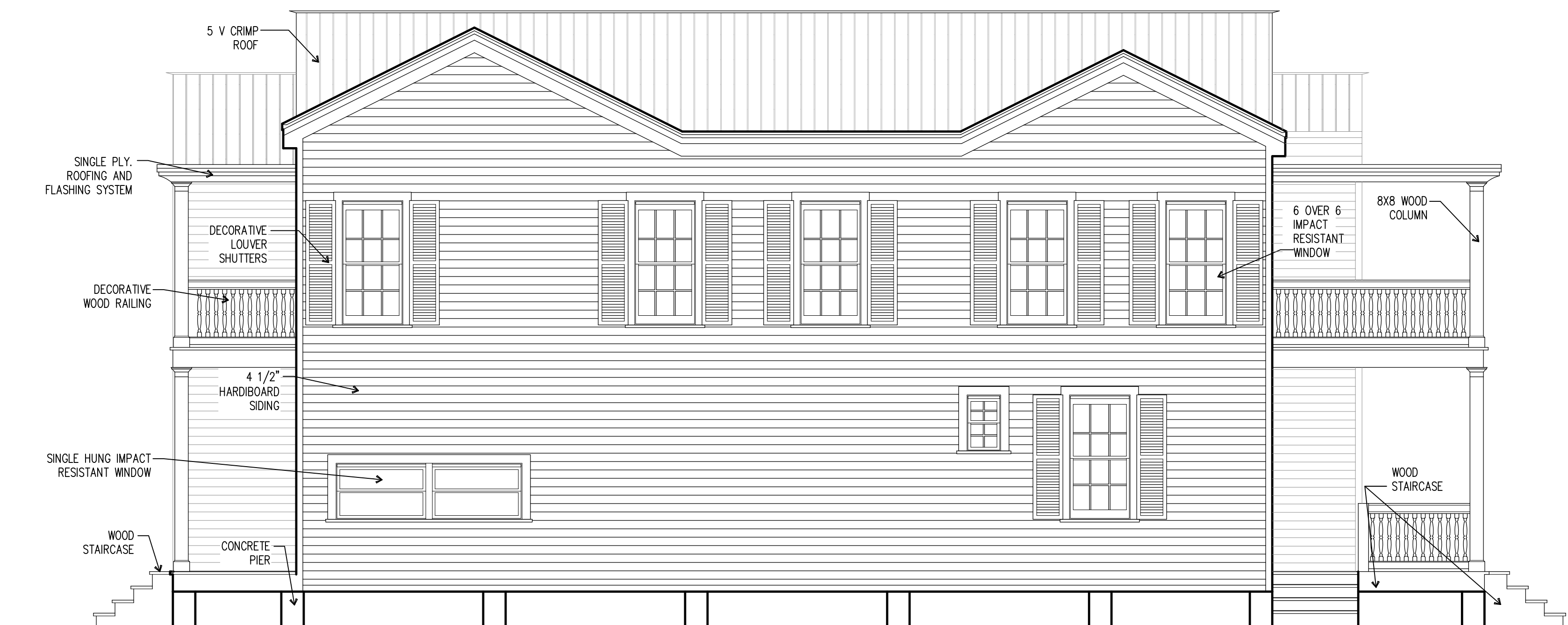
2 UNIT A WEST ELEVATION SCALE: 1/4" = 1'-0"
