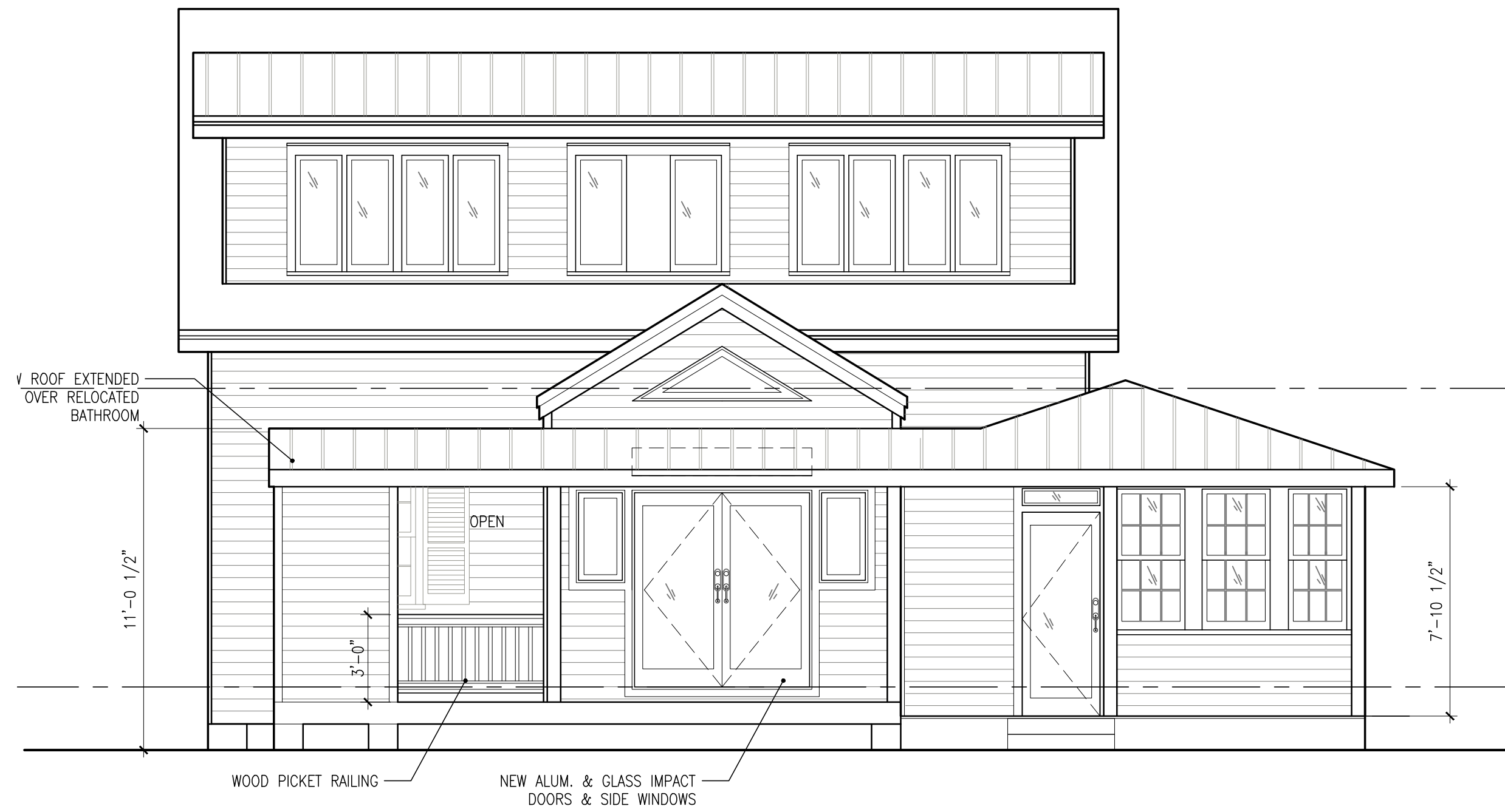
1 A3.1 EAST ELEVATION SCALE: 1/4"=1'-0"
