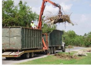
areas on the side of the street. If the crew is working in a high traffic area then this method will not be incorporated – rather the staging will be done completely on one side then staged completely on the other side. When the Knuckleboom loader encounters material difficult to handle (such as chunk wood), the Frontend loader will assist in performing the loading.
