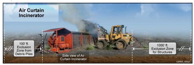
The Air Curtain will be operated at least 100 feet from any stockpile of debris and at least 1,000 feet from any occupied structure. Prior to removal of ash debris from the air curtain incinerator pit, the material will be wetted. Ash stockpiles will be at least 100 feet away from any debris stockpiles.
