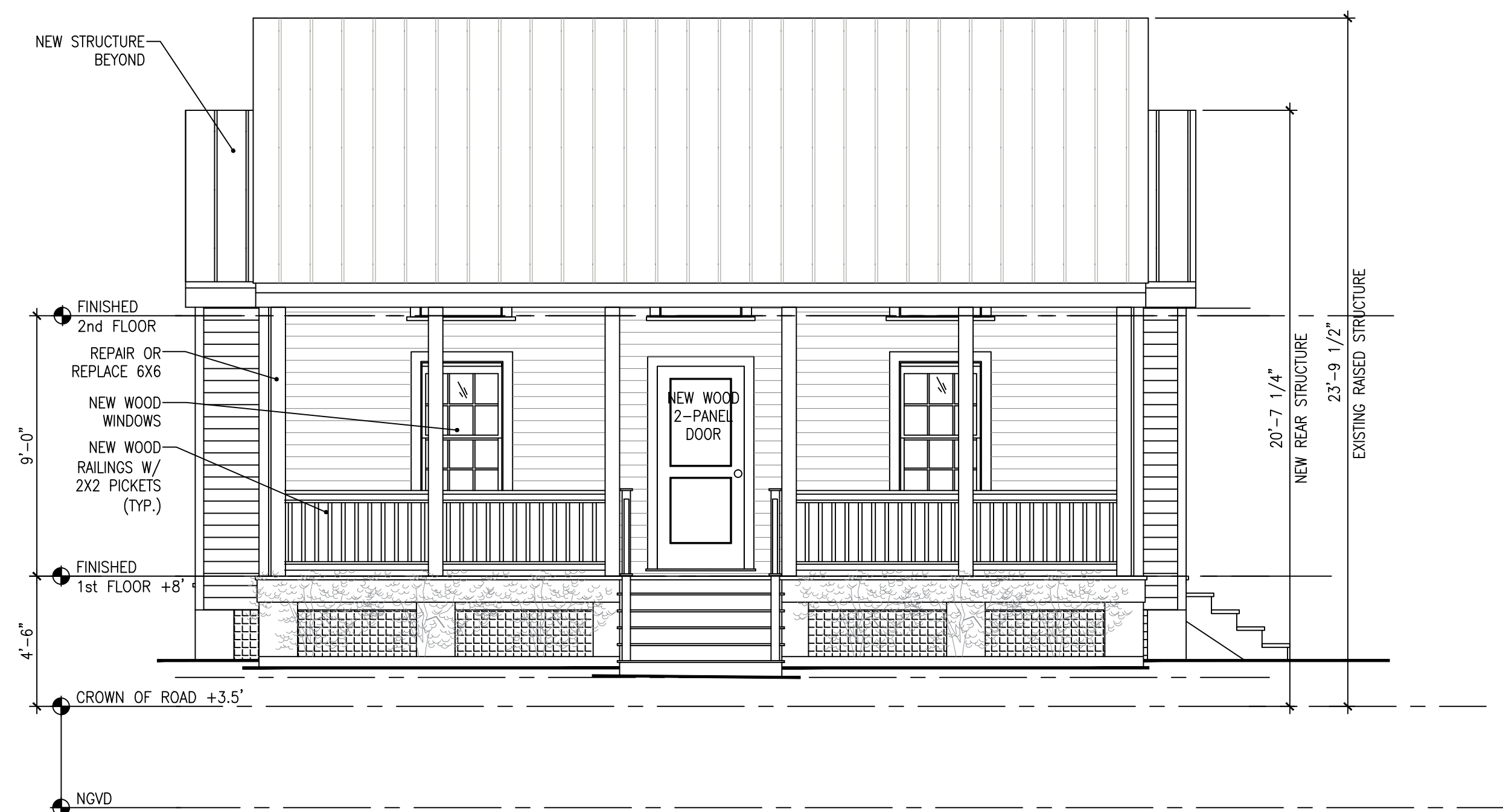
1 FRONT ELEVATION SCALE: 1/4"=1'-0" A31
