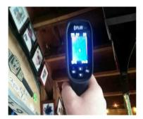
**Location:** Lounge **System:** Interior **Condition:** WET Ceiling Stain Roof Leak **Explanation:** A stain on a ceiling surface is observed to test high for moisture content using moisture meters or thermal imaging camera. The source of the moisture intrusion is suspected to be from an active roof leak.
