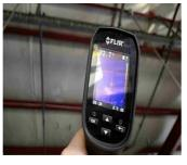
**Location:** Lounge **System:** Interior **Condition:** WET Ceiling Stain Roof Leak **Explanation:** A stain on a ceiling surface is observed to test high for moisture content
