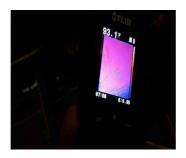
**Location:** Storage **System:** Interior **Condition:** WET Ceiling Stain Roof Leak **Explanation:** A stain on a ceiling surface is observed to test high for moisture content using moisture meters or thermal imaging camera. The source of the moisture intrusion is suspected to be from an active roof leak.
