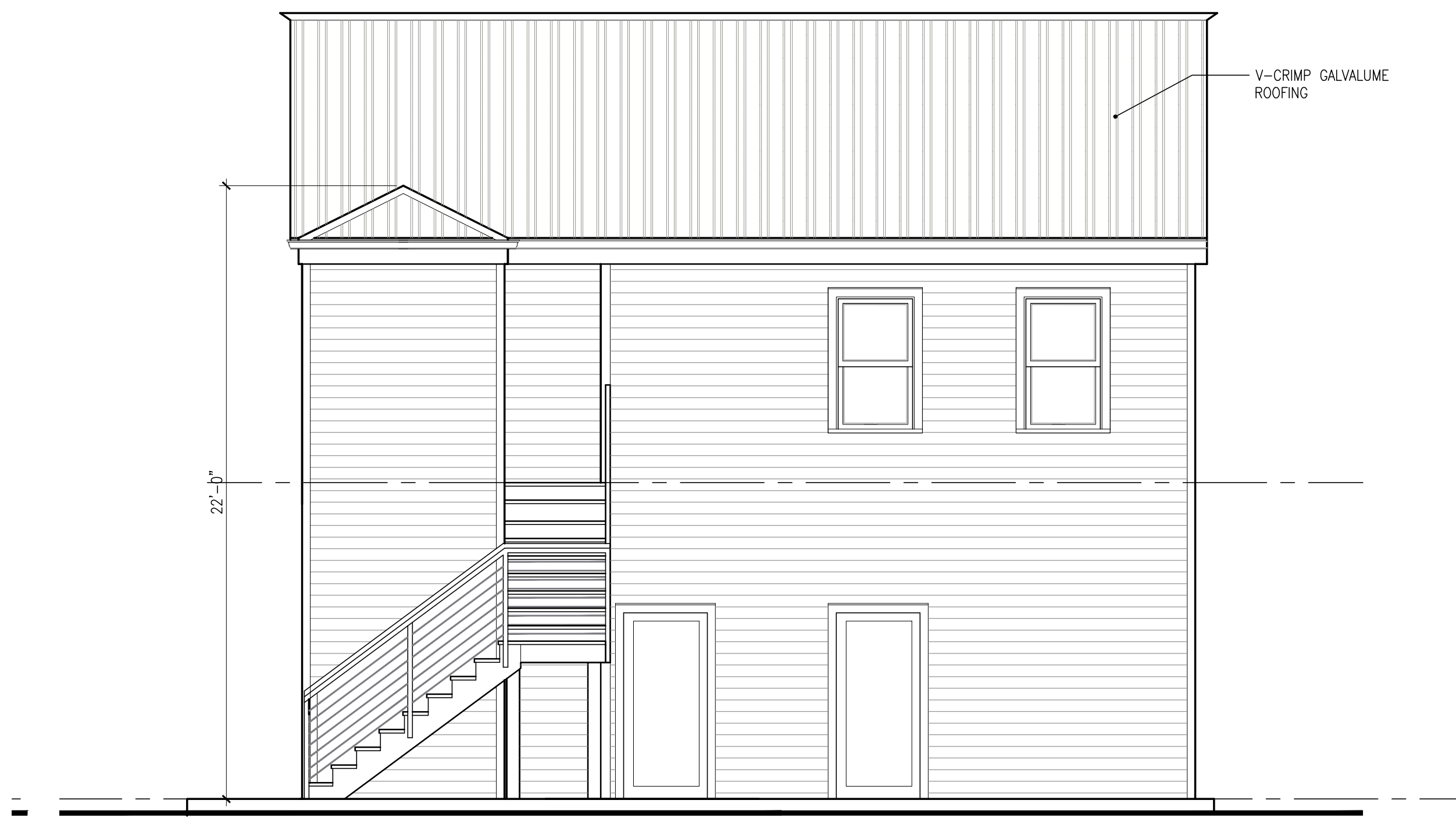
3 A3.1 COMMERCIAL - SOUTH ELEVATION SCALE: 1/4"=1'-0"
