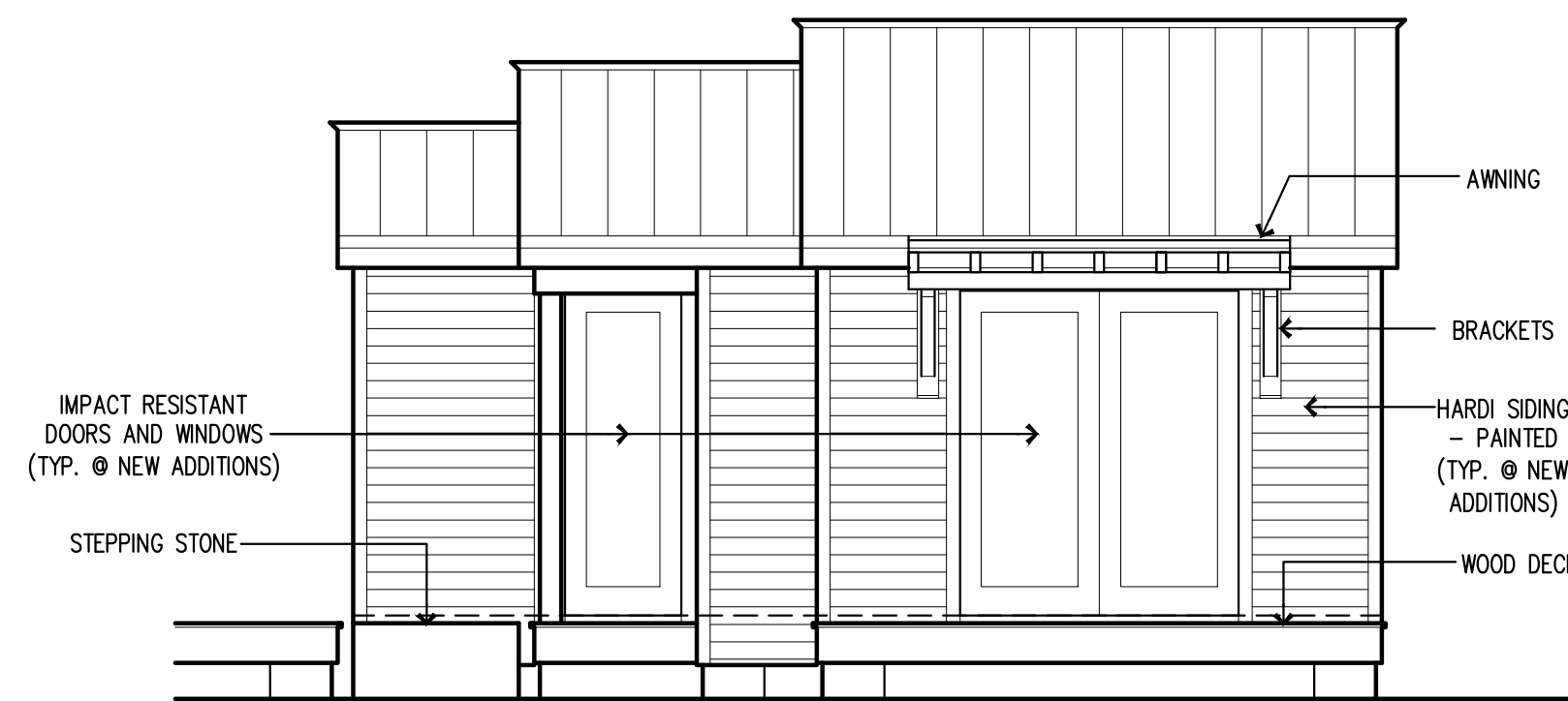
PROPOSED EAST SIDE ELEVATION OF COTTAGE 1/4"=1'-0"
