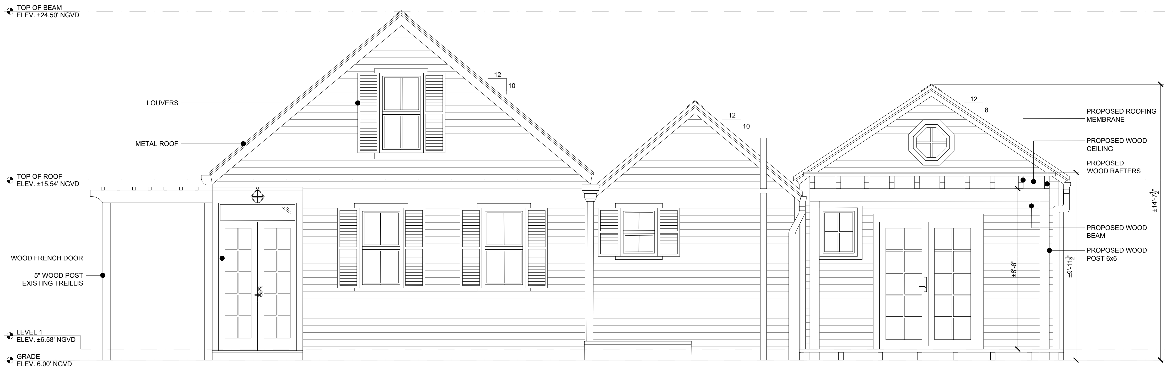
PROPOSED REAR ELEVATION SCALE: 3/8" = 1'-0"
