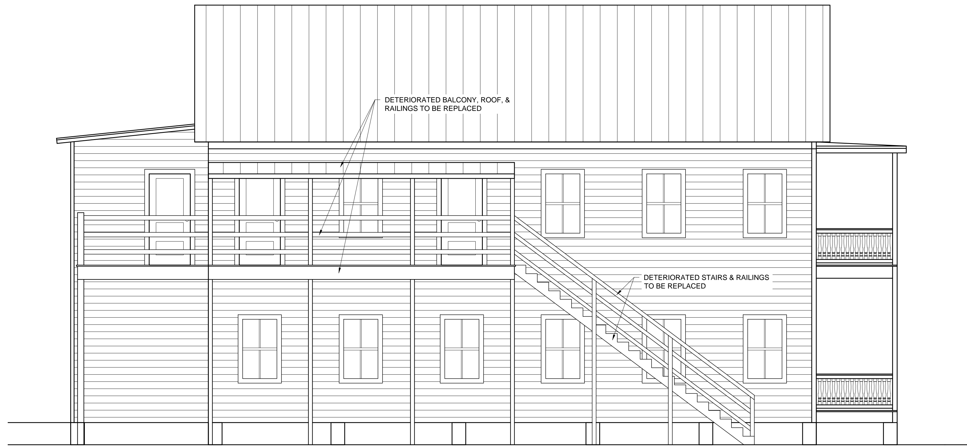
EXISTING SIDE ELEVATION
