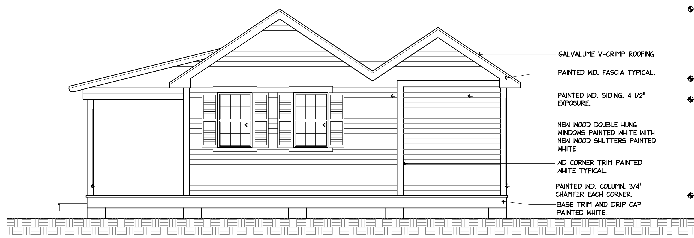
1 BUILDING #3 (STUDIO) NORTH ELEVATION SCALE: 1/4"=1'-0"
