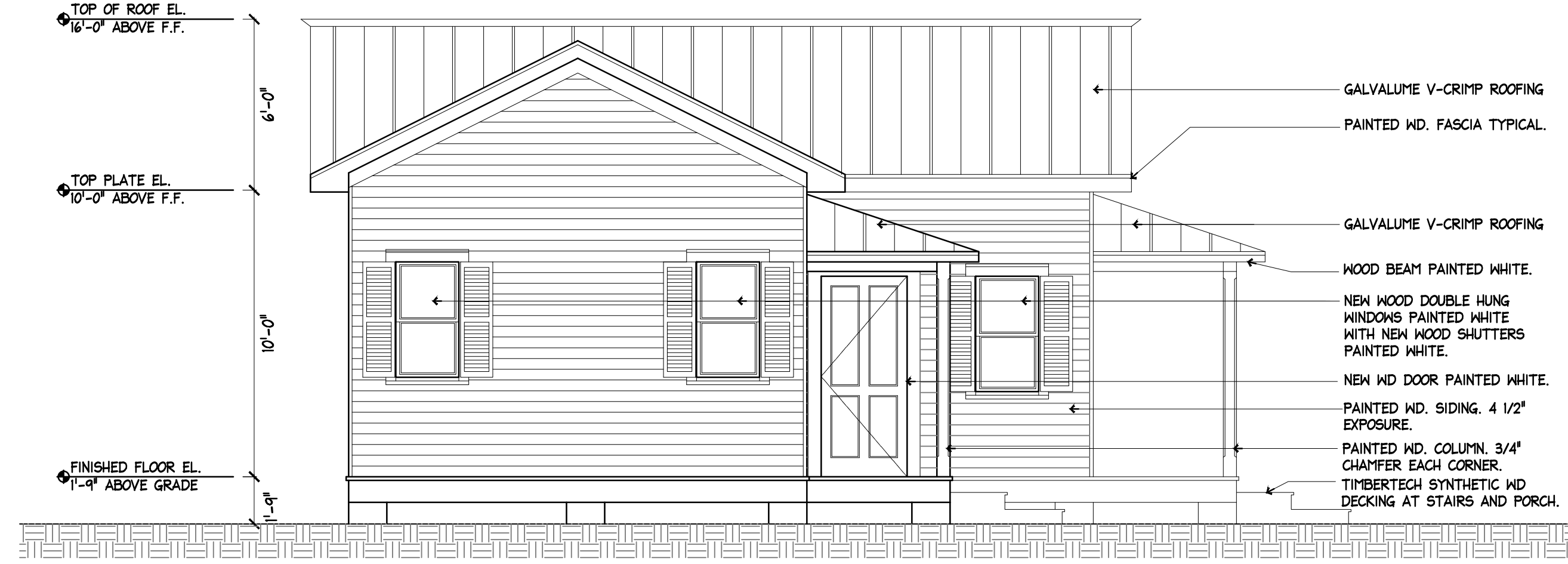
1 BUILDING #2 (COTTAGE) EAST ELEVATION SCALE: 1/4"=1'-0"
