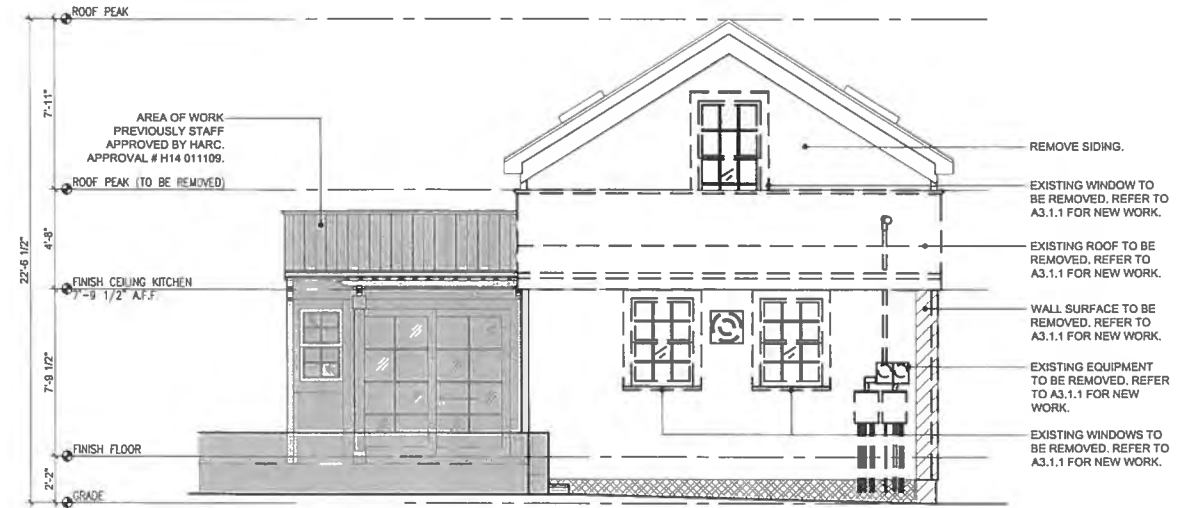
3 DEMOLITION SOUTH ELEVATION SCALE: 1/4"=1'-0"
