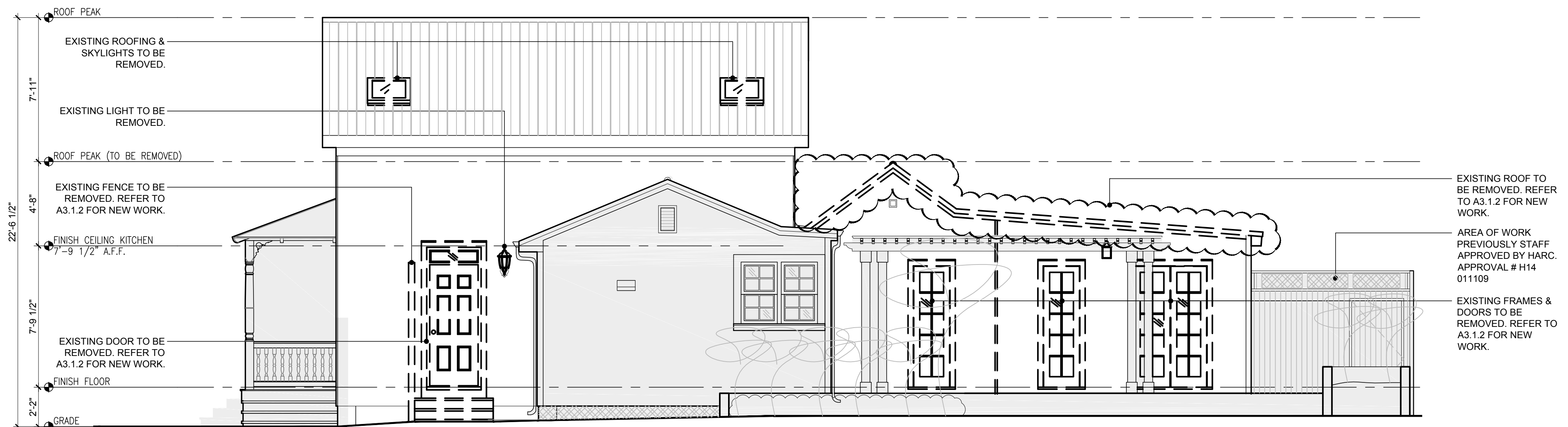
1 DEMOLITION WEST ELEVATION SCALE: 1/4"=1'-0" GRAPHIC SCALE: 1/4" = 1'-0"
