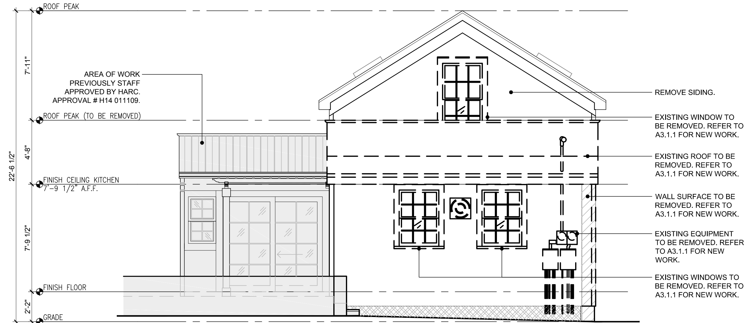
3 DEMOLITION SOUTH ELEVATION SCALE: 1/4"=1'-0" GRAPHIC SCALE: 1/4" = 1'-0"
