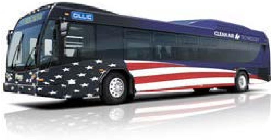
Gillig Hybrid Electric Clean Diesel (Low Sulfur) Bus
