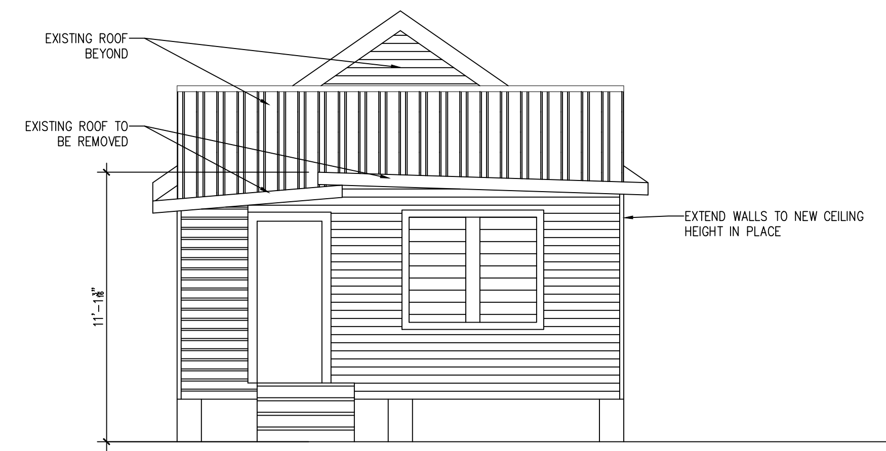
1 EXISTING REAR ELEVATION CS-1 SCALE: 1/4"= 1'-0"
