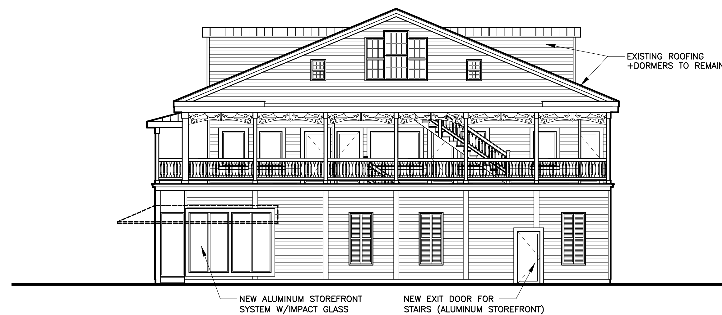
2 A-5 PROPOSED SIDE ELEVATION - 2 SCALE: 1/8"=1'-0"
