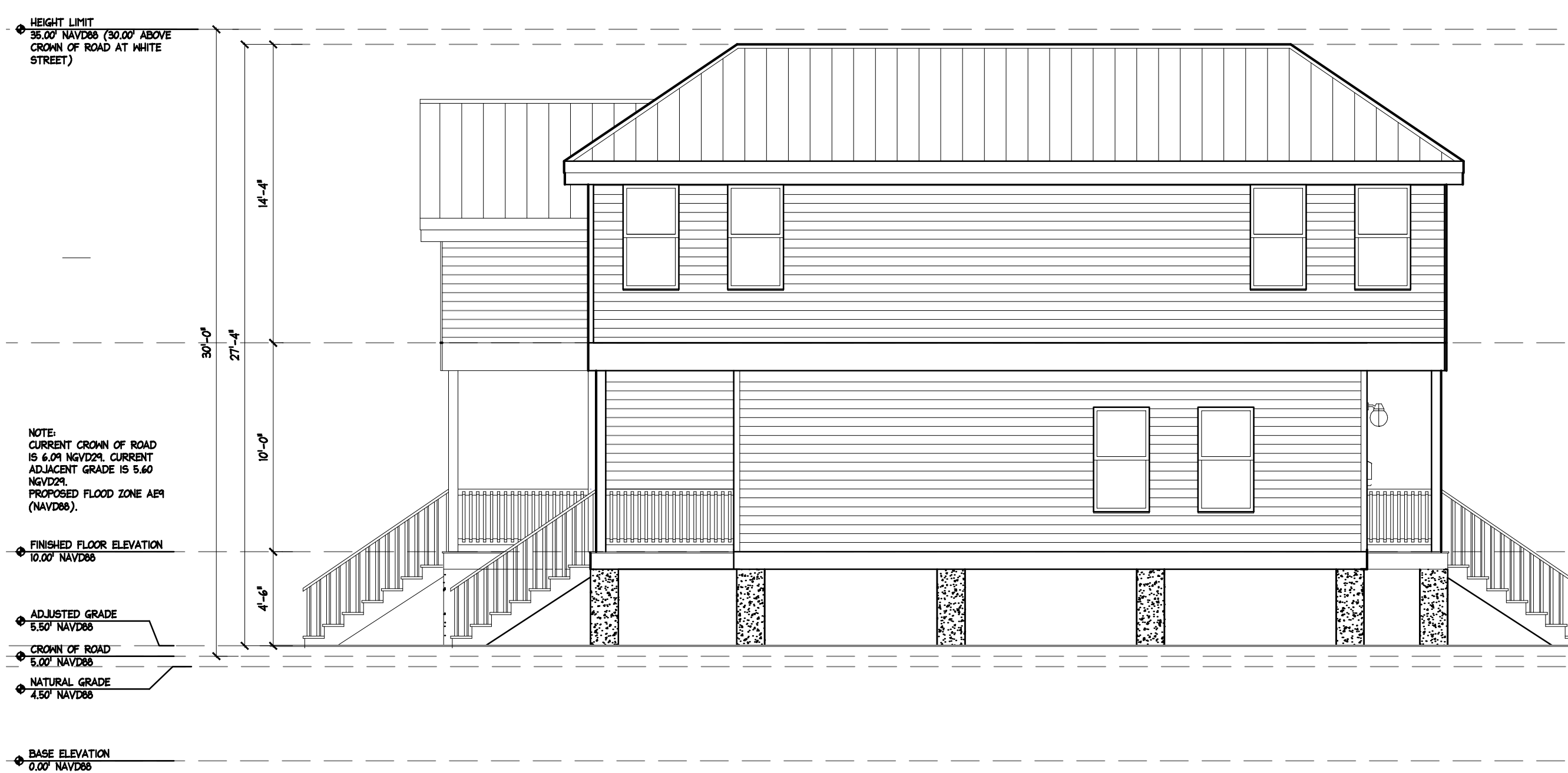
2 QUINTUPLEX SIDE ELEVATION (SITE #9) SCALE: 3/16"=1'-0"
