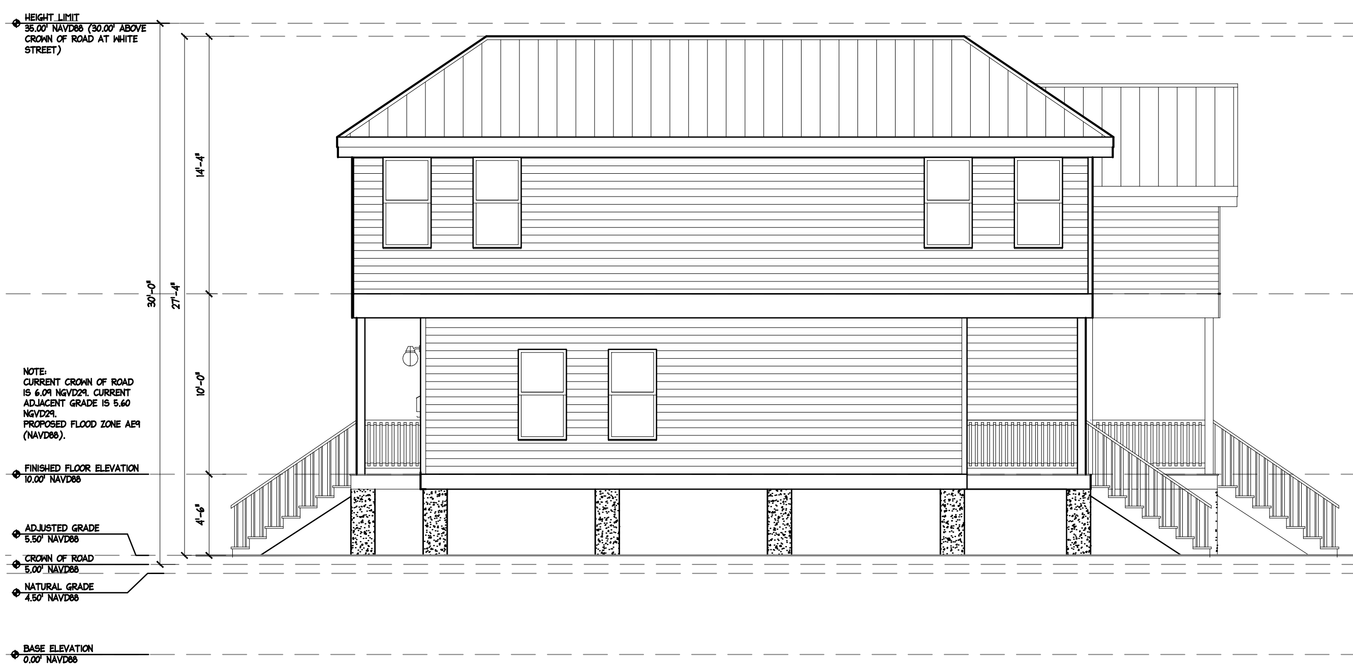
4 QUINTUPLEX SIDE ELEVATION (SITE #9) SCALE: 3/16"=1'-0"
