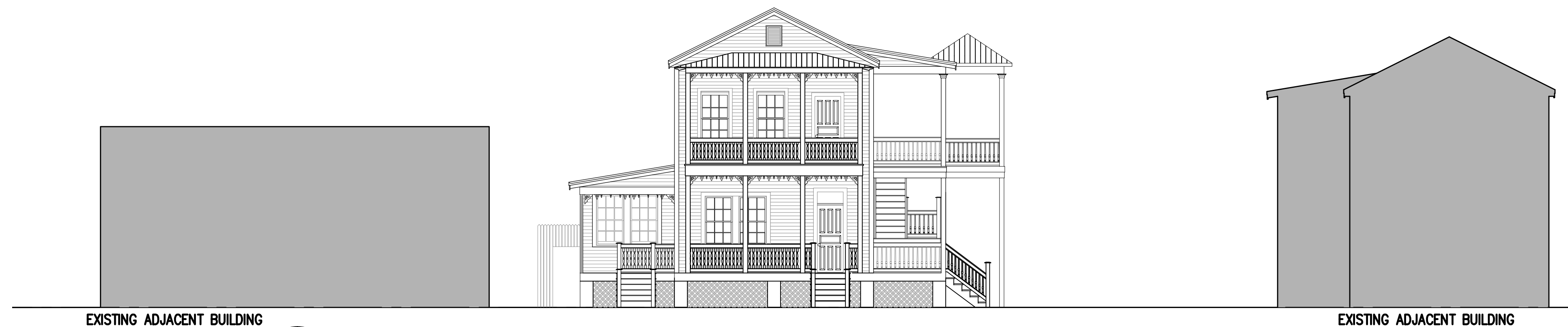
5 PROPOSED FRONT ELEVATION W/ADJACENT PROPERTIES (from Eisenhower Dr.) A-2 SCALE: 1/8" = 1'-0"
