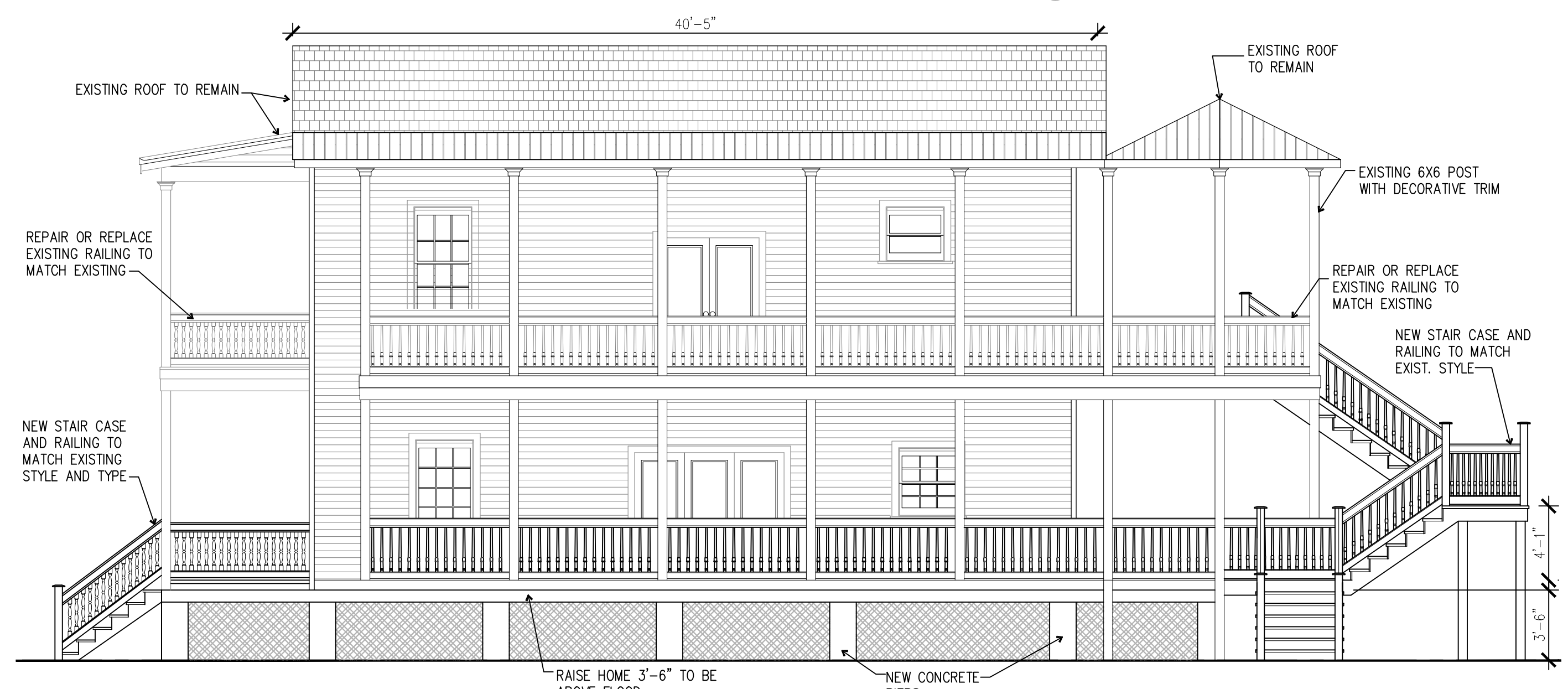
4 PROPOSED NORTH SIDE ELEVATION A-2 SCALE: 3/16" = 1'-0"
