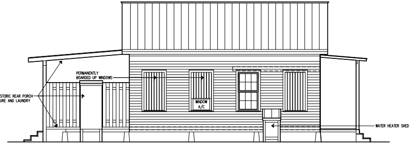
EXISTING SOUTH SIDE ELEVATION 1/4"=1'-0"
