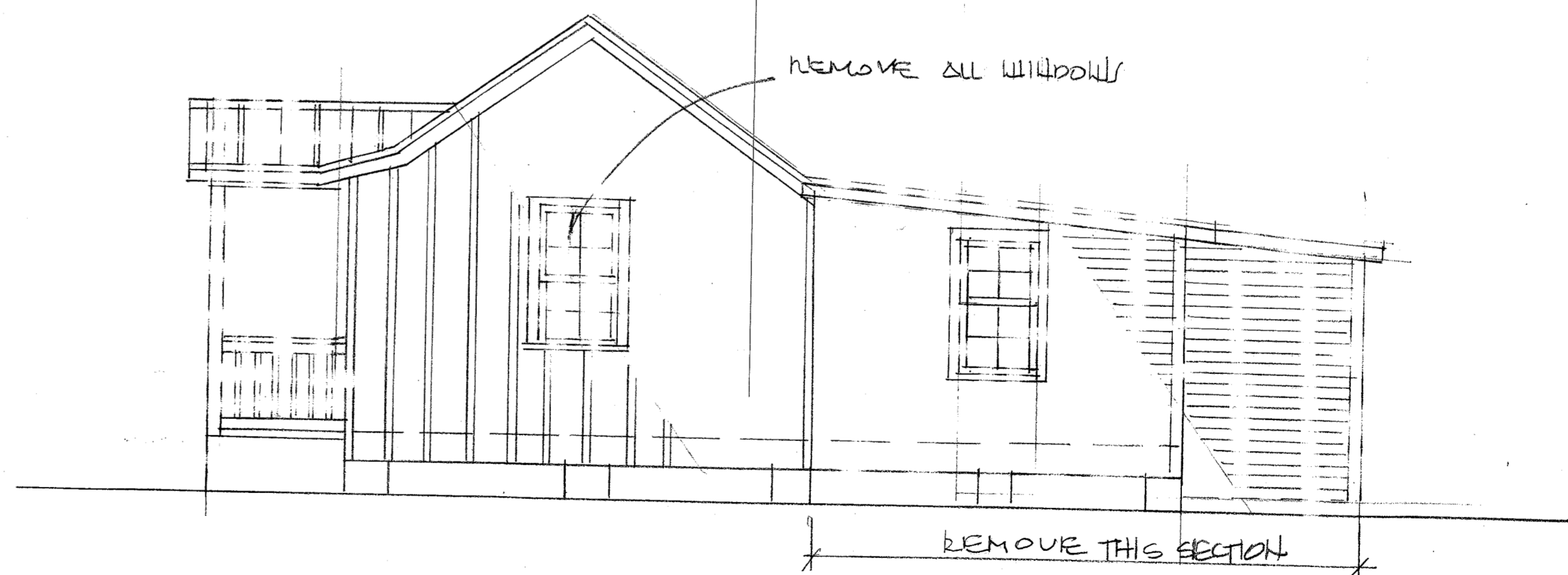
EXISTING/DEMOLITION SIDE ELEVATION (SOUTH ELEVATION) - 1/4" = 1'-0"
