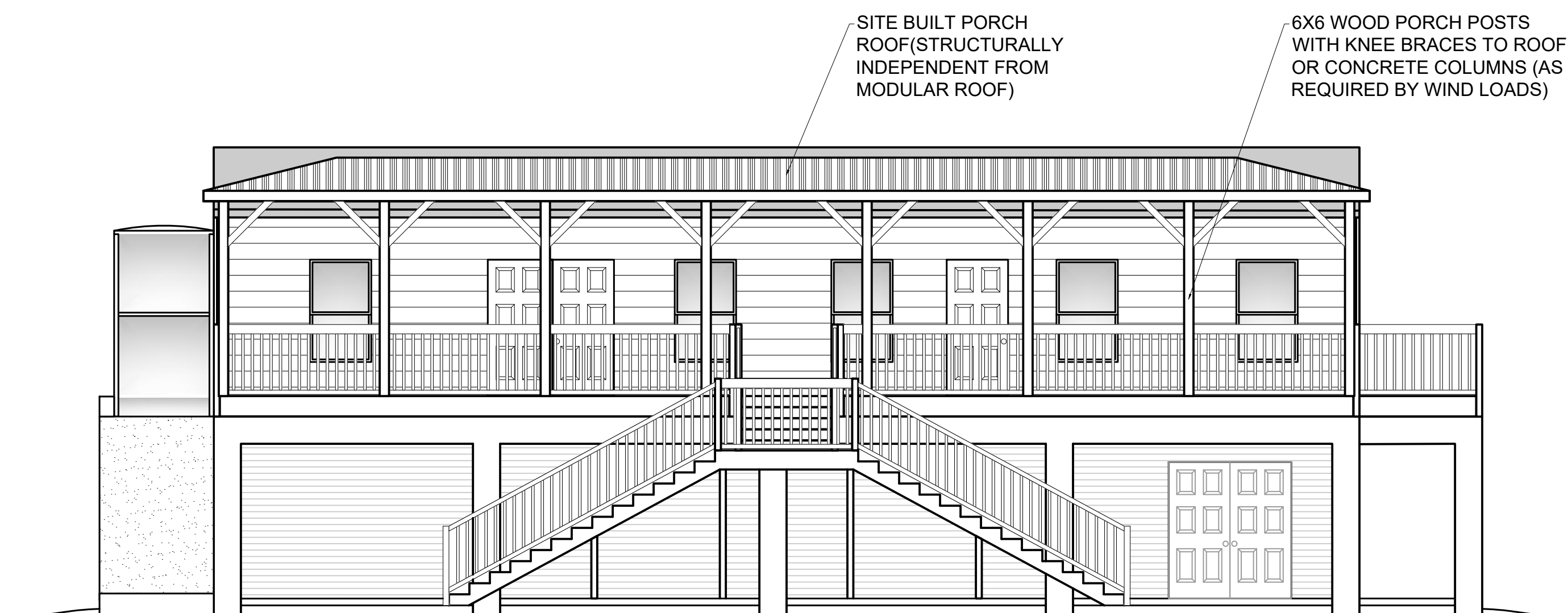
WEST ELEVATION - PROPOSED
