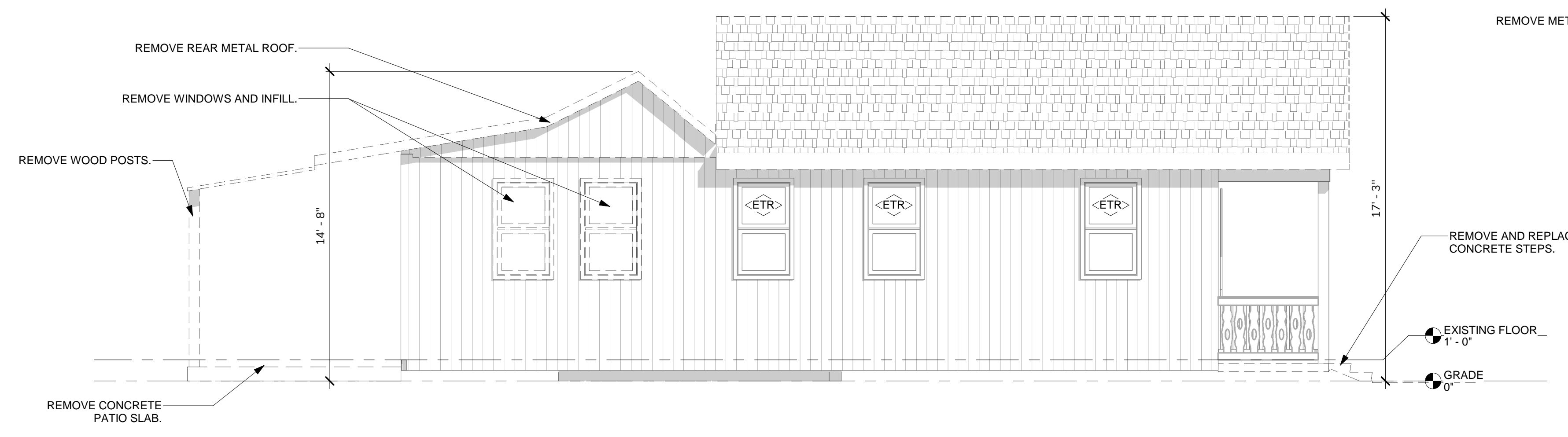
2 DEMOLITION EAST ELEVATION SCALE: 1/4" = 1'-0"
