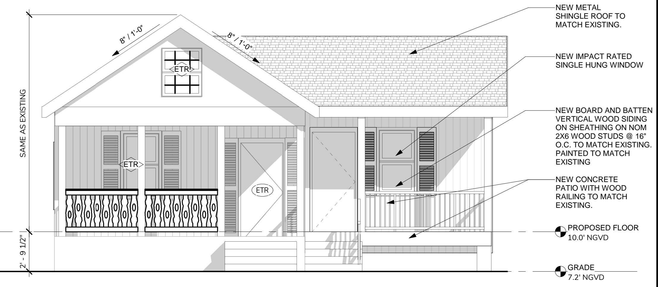
3 NORTH (FRONT) ELEVATION SCALE: 1/4" = 1'-0"
