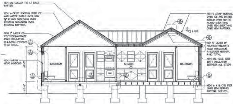
6 SECTION LOOKING NORTH SCALE: 1/4" = 1'-0"
