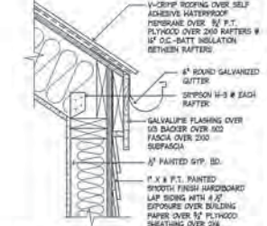
11 ROOF EAVE SCALE: 1/2" = 1'-0"
