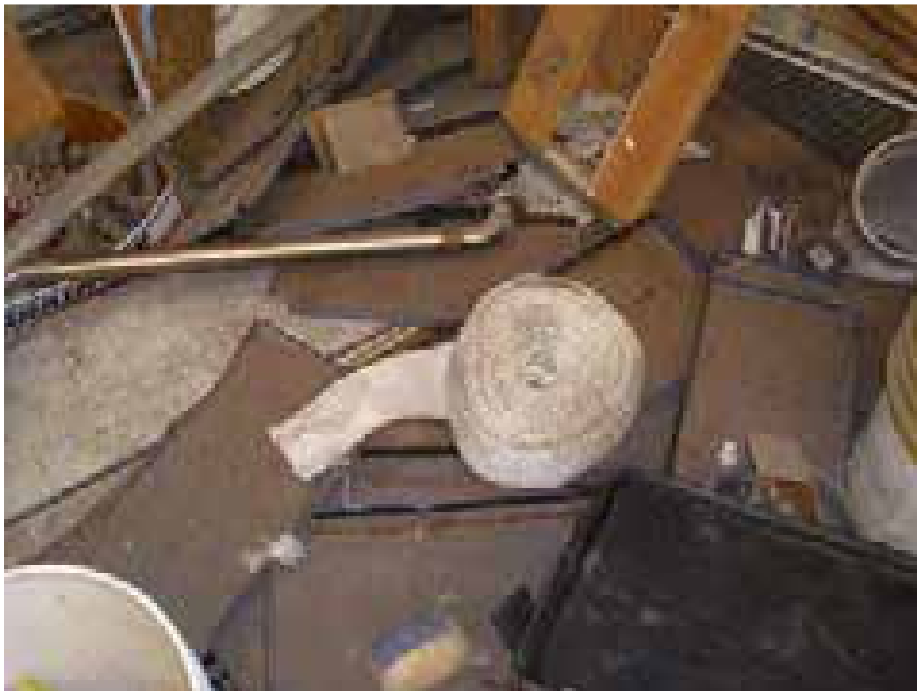
Photo 4: Typical nonACM white roll insulation sampled during this inspection.
