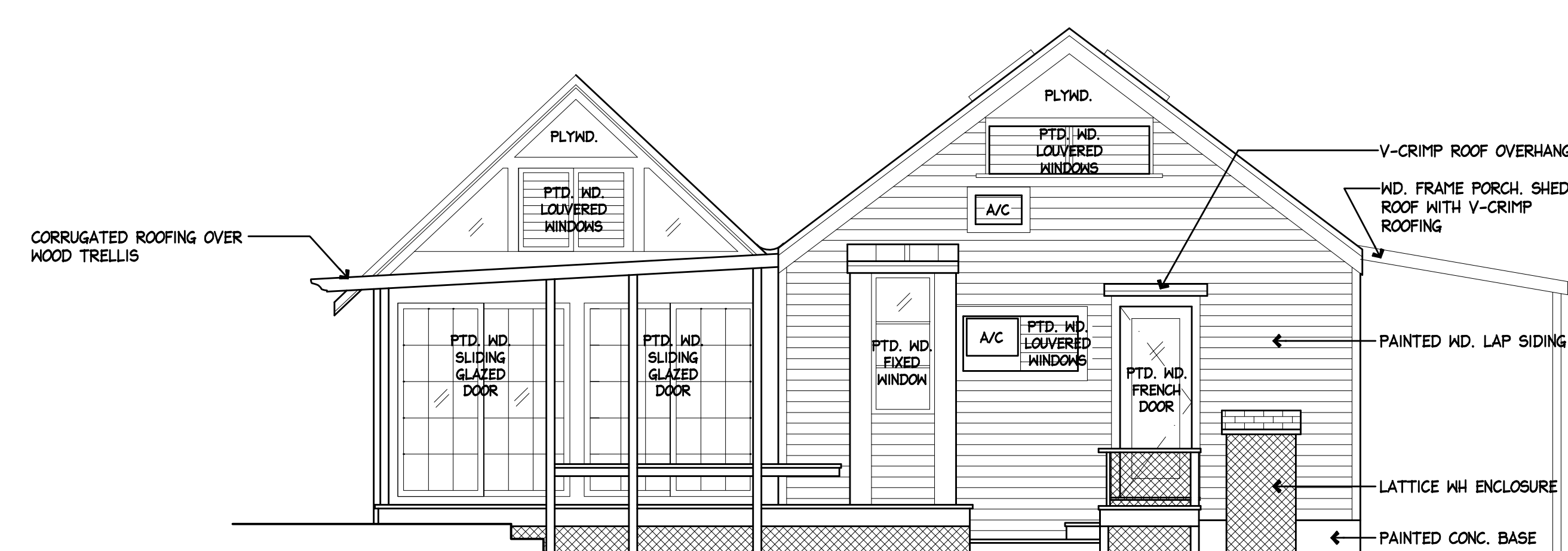
3 EXISTING REAR (SOUTH) EXTERIOR ELEVATION EX2 SCALE: 1/4"=1'-0"
