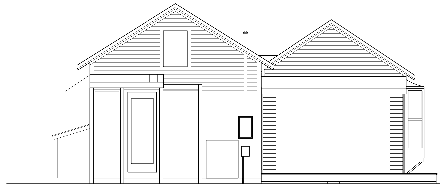
EXISTING REAR ELEVATION – NORTH 1/4"=1'-0"
