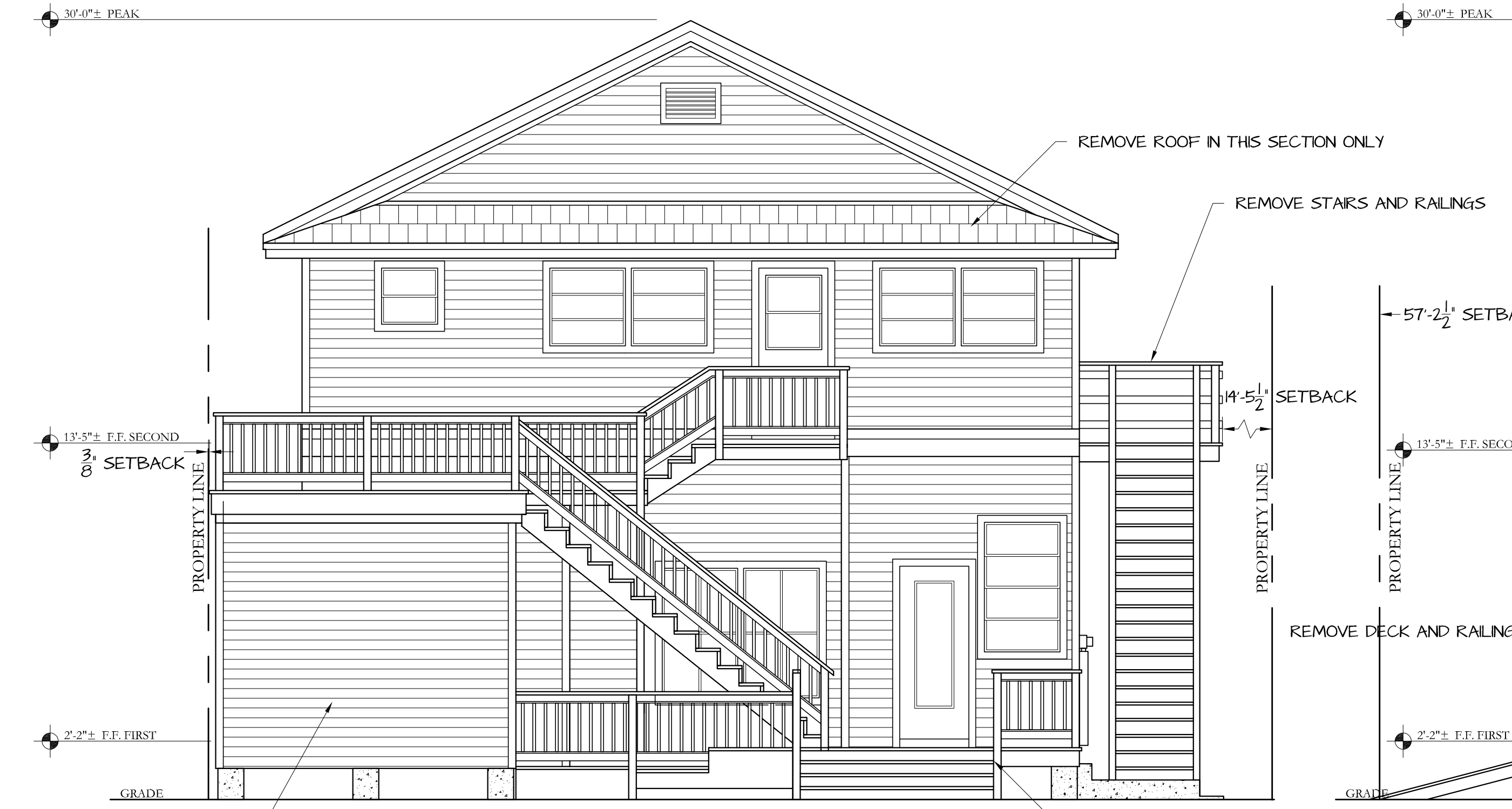
NORTH ELEVATION (EXISTING) 1/4" = 1'-0"
