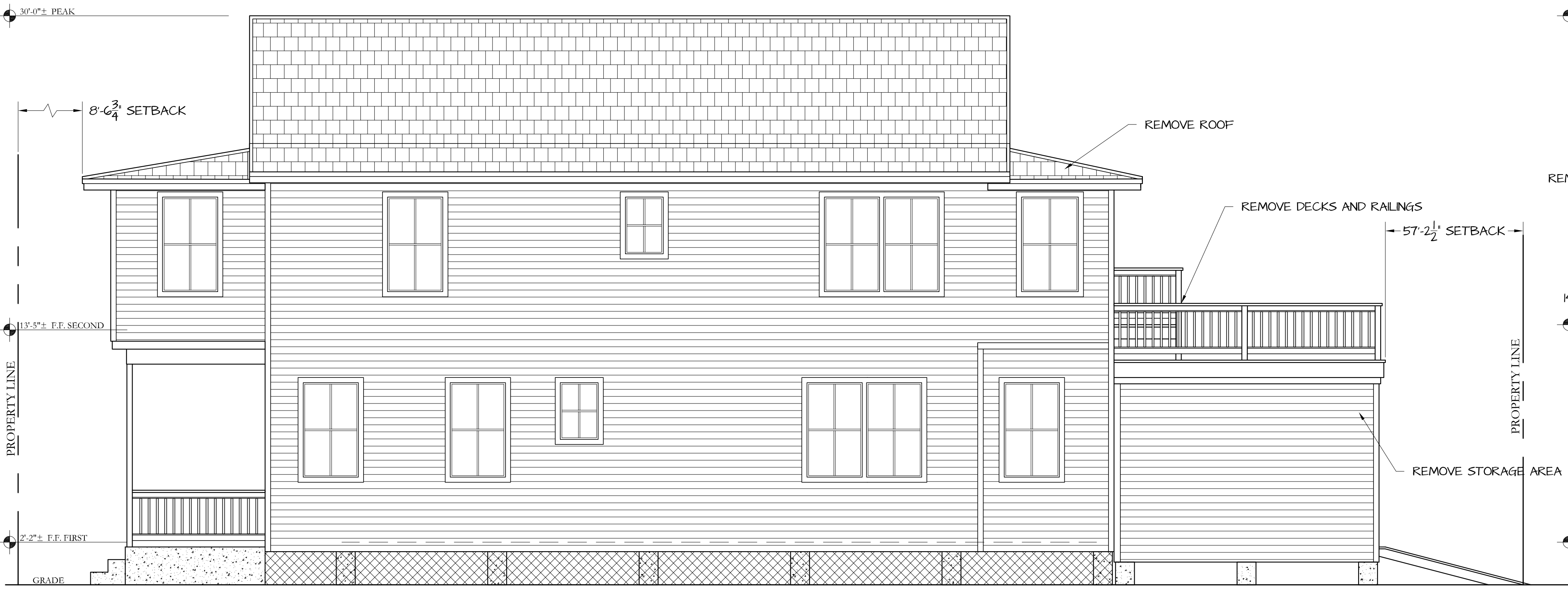
EAST ELEVATION (EXISTING) 1/4" = 1'-0"
