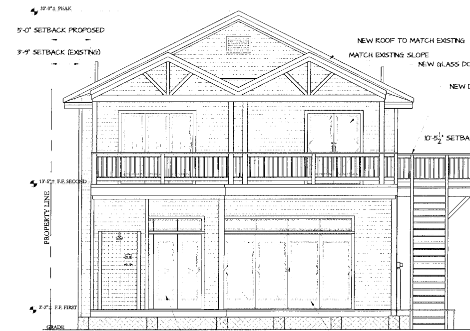
NORTH ELEVATION (PROPOSED) 1/4" = 1'-0"
