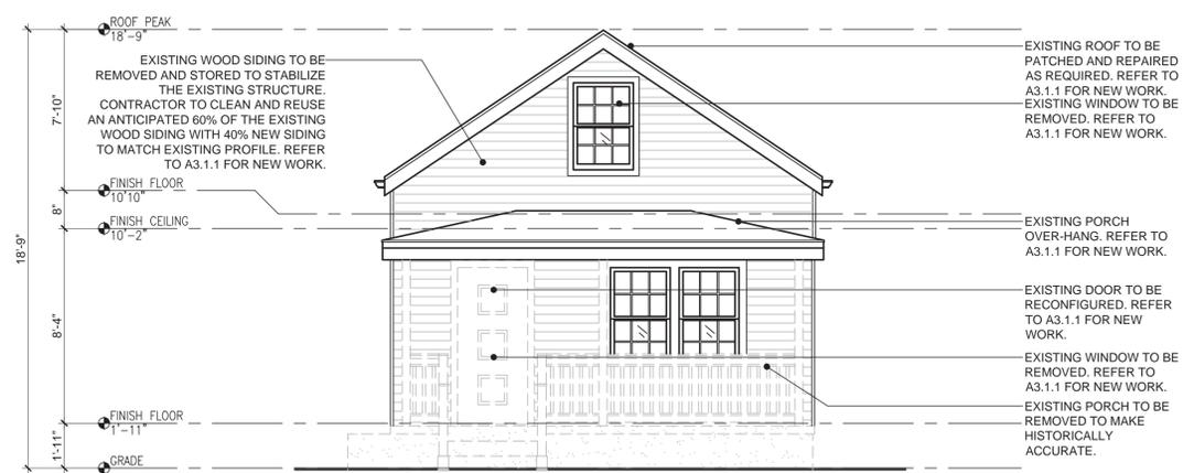
**1** DEMOLITION SOUTH ELEVATION
