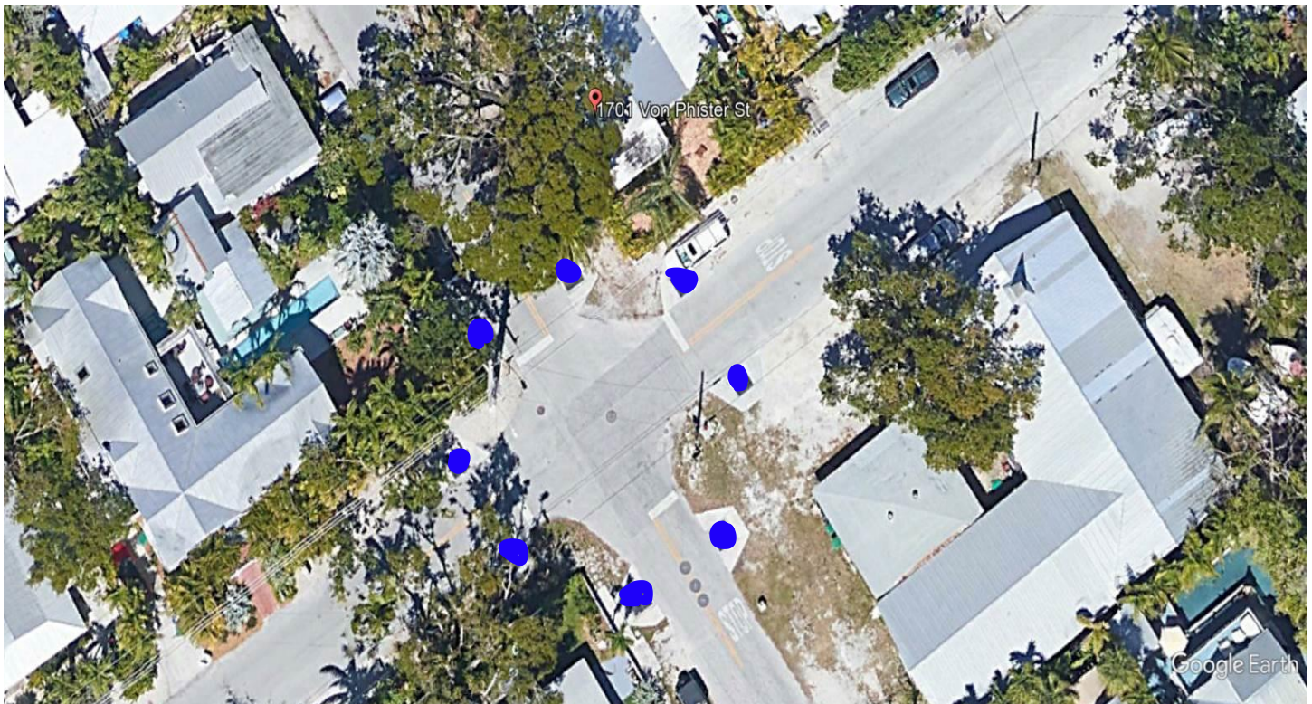
Aerial photo showing locations of street drains.
