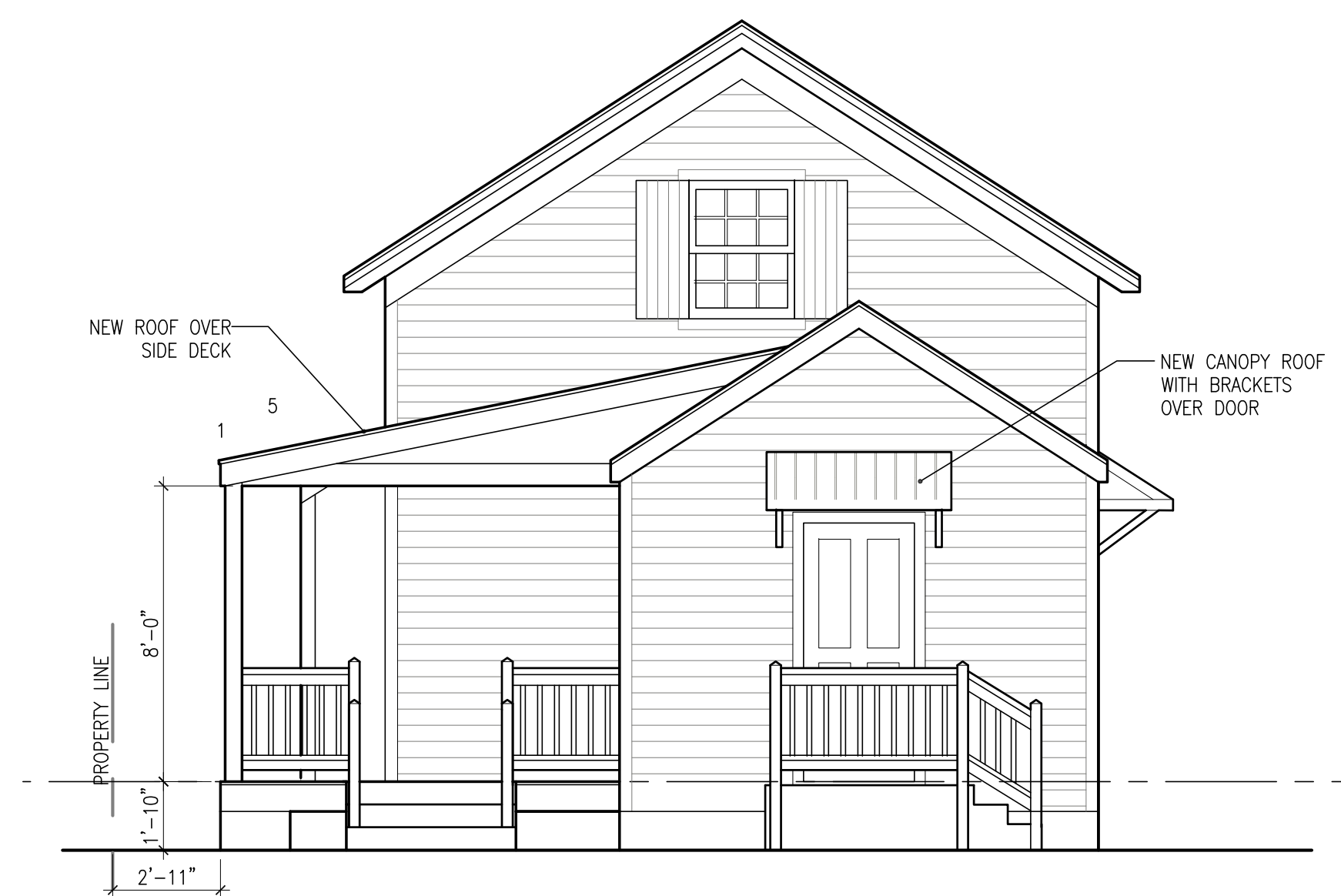
2 A2 PROPOSED REAR ELEVATION SCALE: 1/4"=1'-0"
