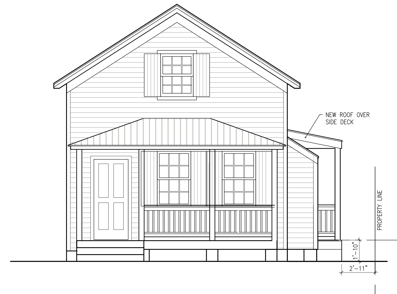
3 A2 PROPOSED FRONT ELEVATION SCALE: 1/4"=1'-0"
