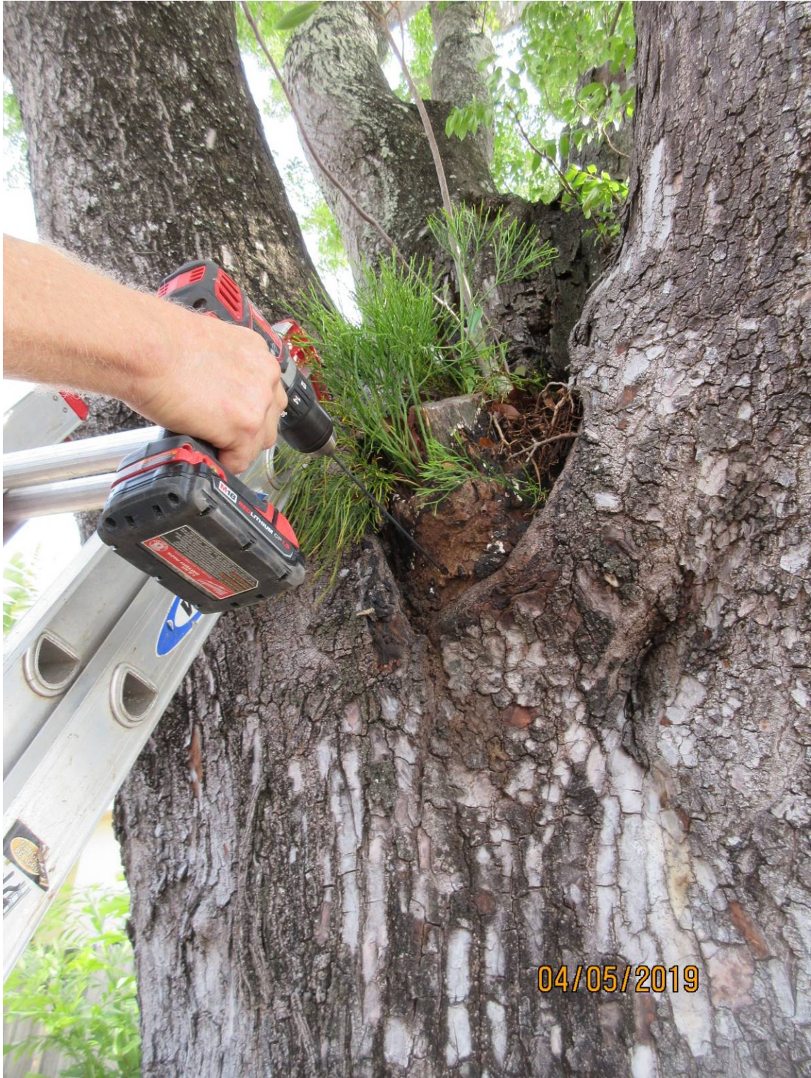
Drill location above- 2" soft then hard wood.
