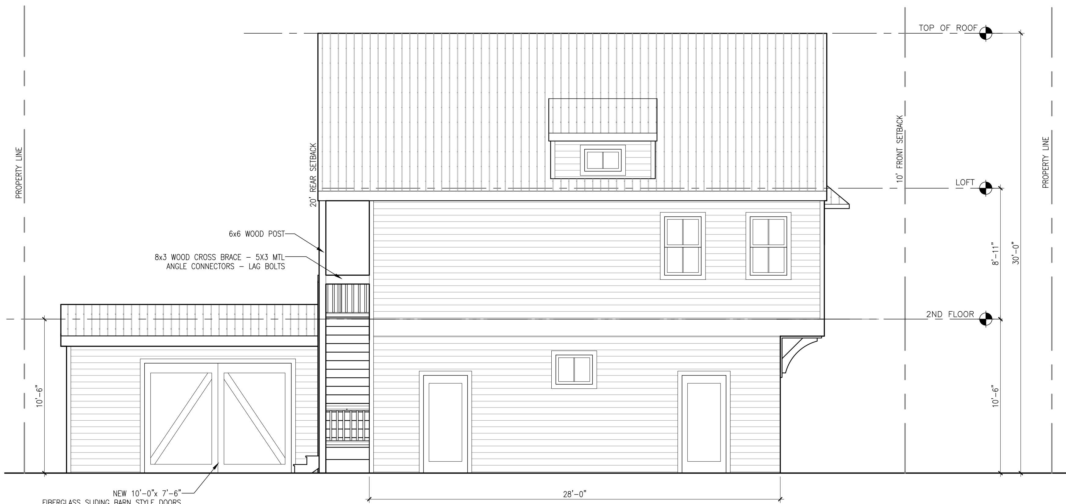
2 WEST ELEVATION A3.1 SCALE: 1/4"=1'-0"
