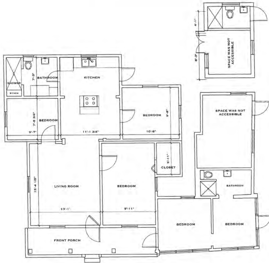
1 EXISTING FIRST FLOOR PLAN EX1.1 SCALE: 1/4" = 1'-0"
