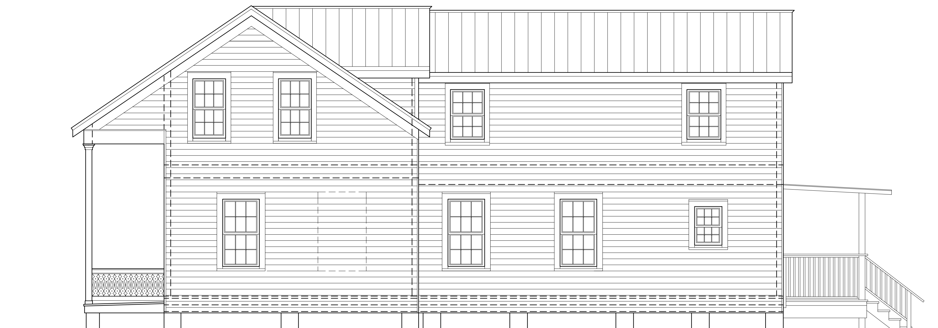
EXISTING SIDE ELEVATION (EAST) - MAIN HOUSE 1/4"=1'-0"
