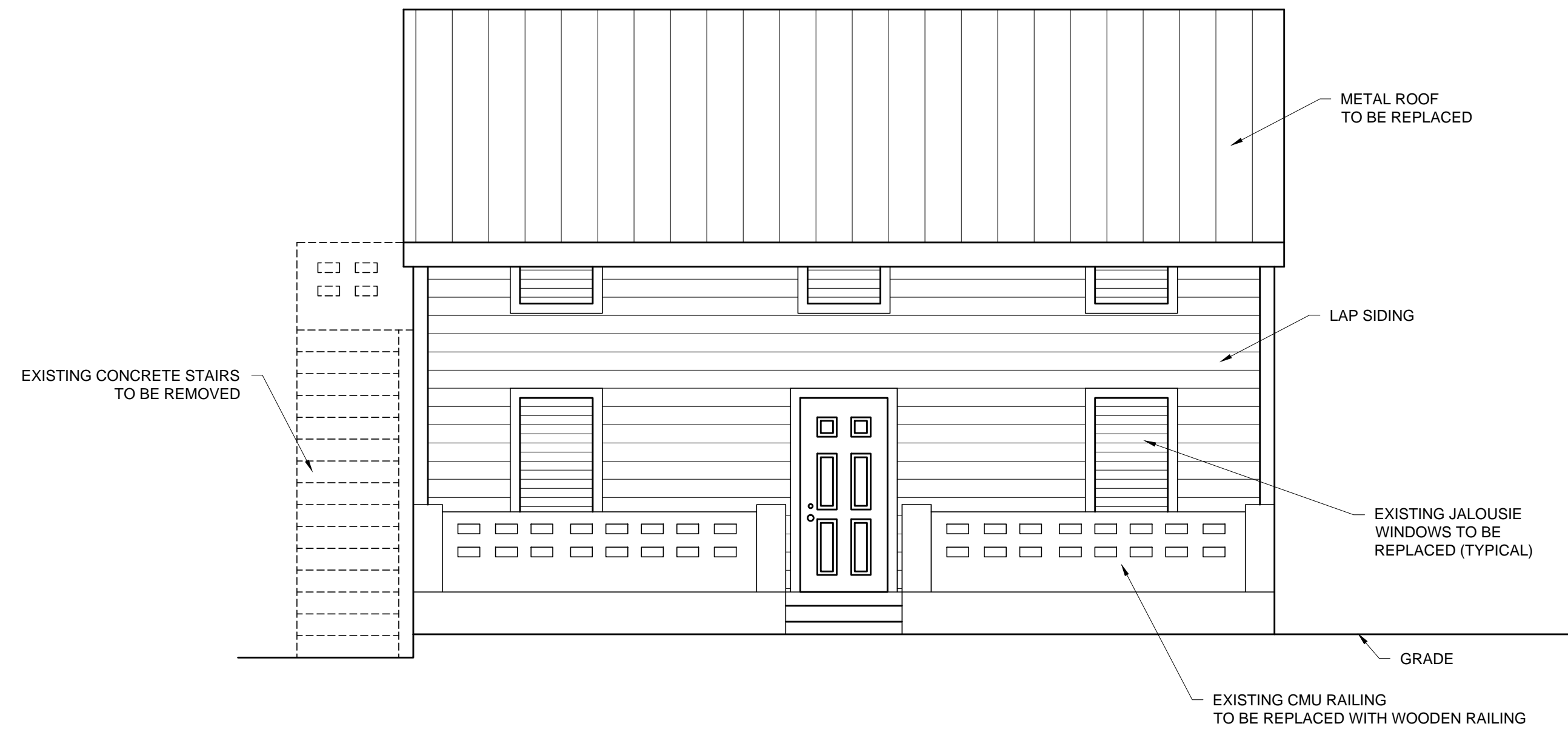
EXISTING SOUTHEAST ELEVATION
