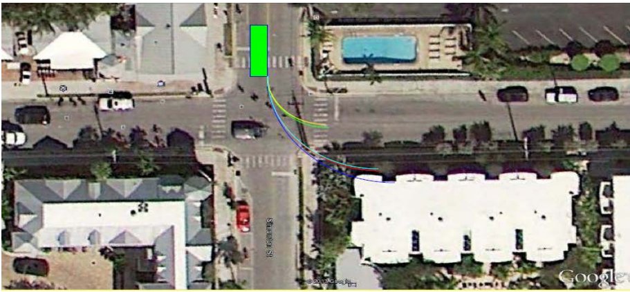
Bus Turning Radii overlaid at the intersection of Simonton and South Street
