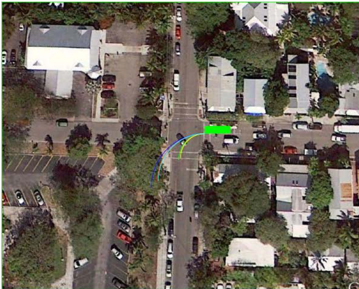
Bus Turning Radii overlaid at the intersection of Eaton and Whitehead Streets
