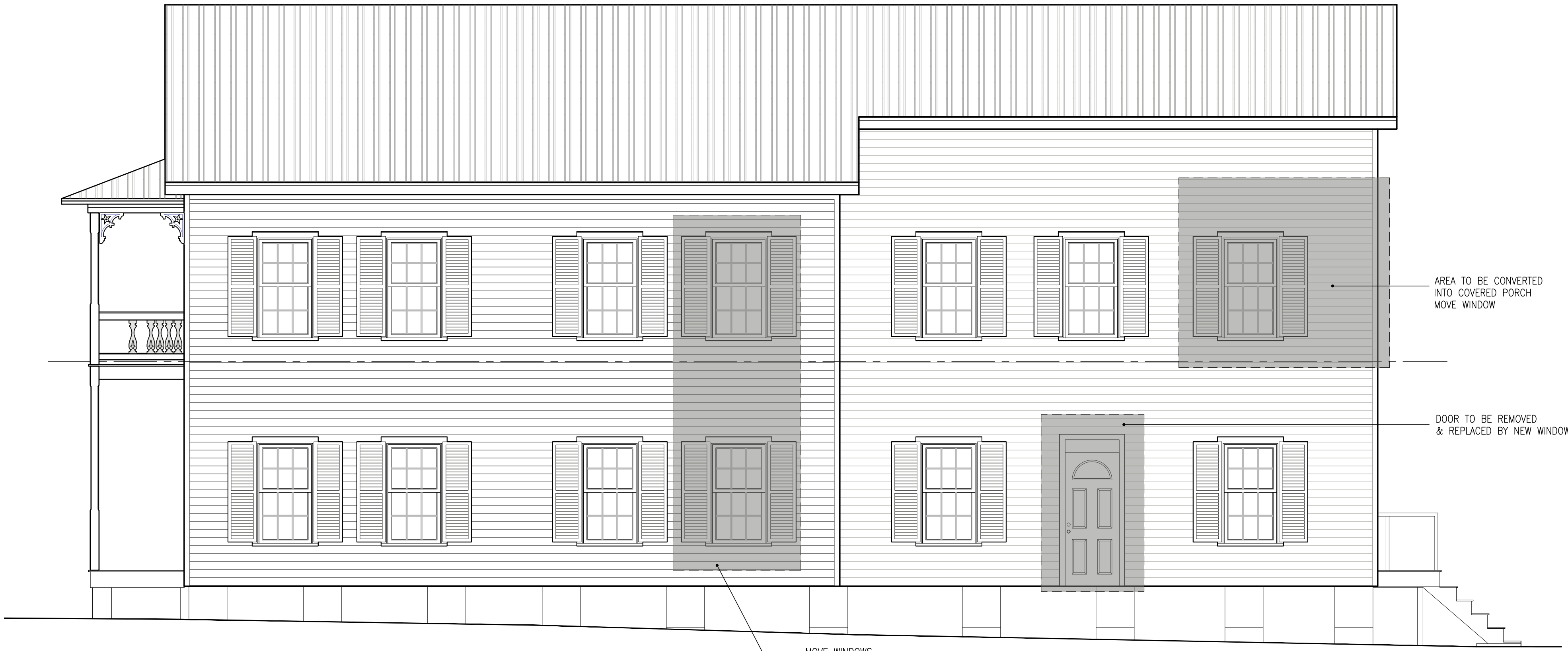
3 EXISTING SOUTH ELEVATION / DEMO AE3.1 SCALE: 1/4"=1'-0"
