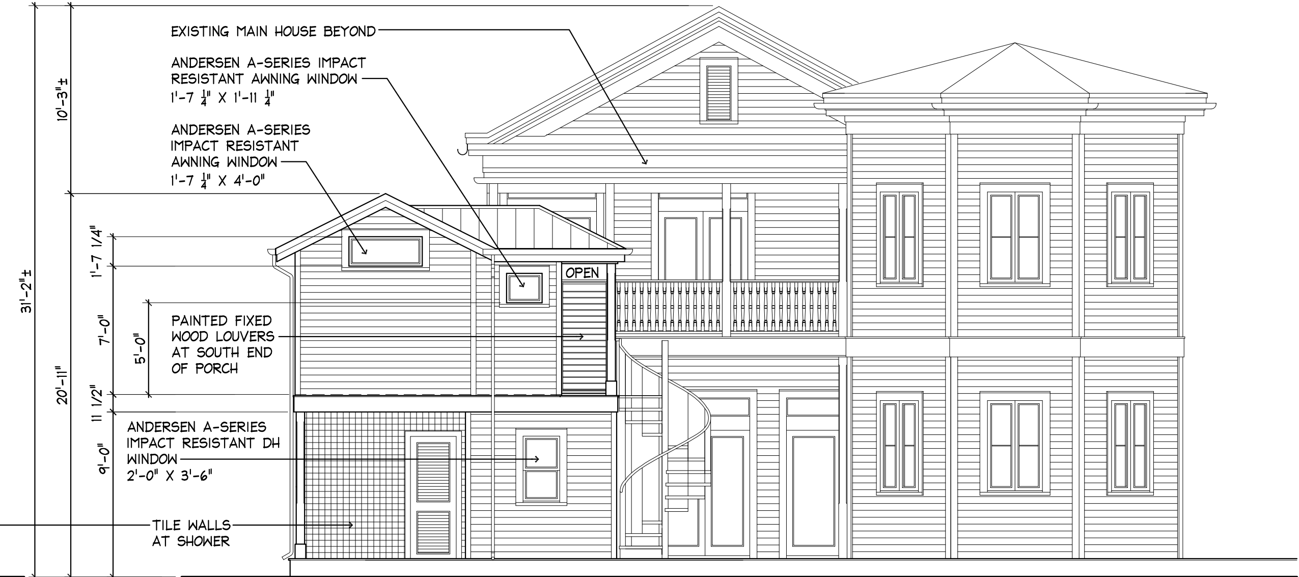
SOUTH ELEVATION (REAR) 3/16"=1'-0"
