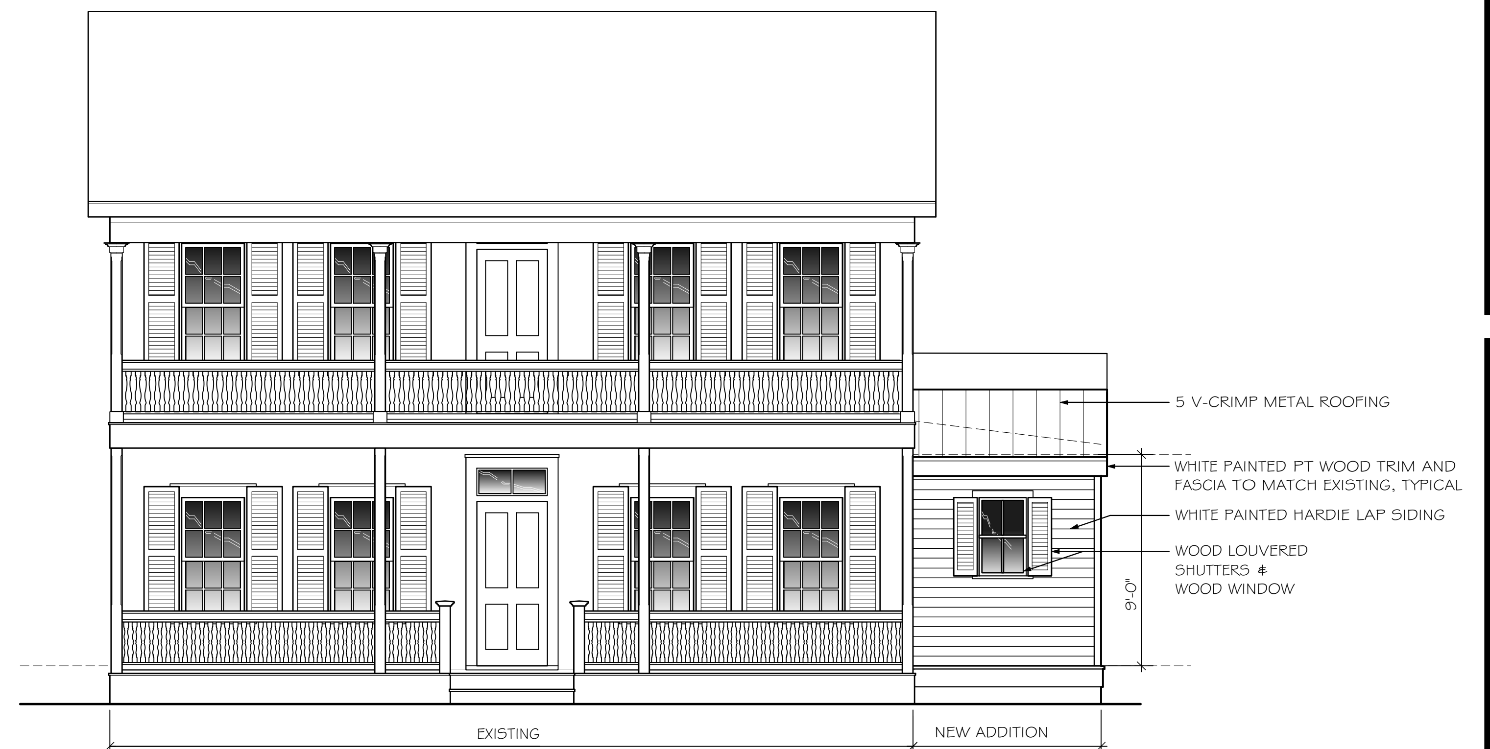
3 Proposed Front Elevation EX-2 1/4" = 1'-0"
